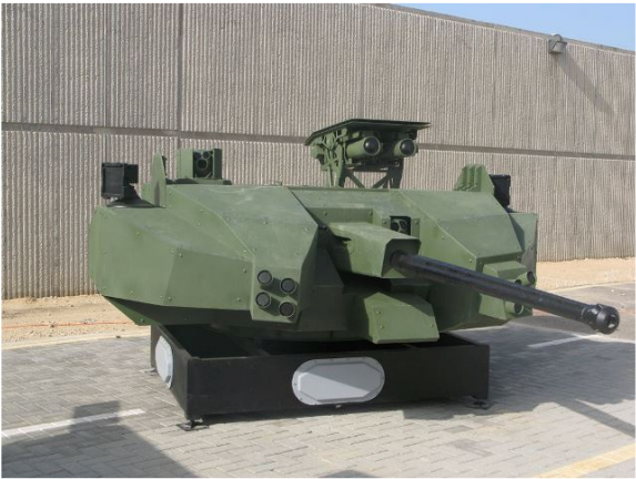
Appearance of a variant of the 30mm Samson turret with the twin Spike missile launcher and the Trophy effectors. In this case, the radars would be mounted on the (Rafael) barge.
