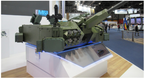
Escribano's RWS Guardian 30 with scale models of the Iron Fist sensors and effectors, exhibited at the recent FEINDEF exhibition (author)
