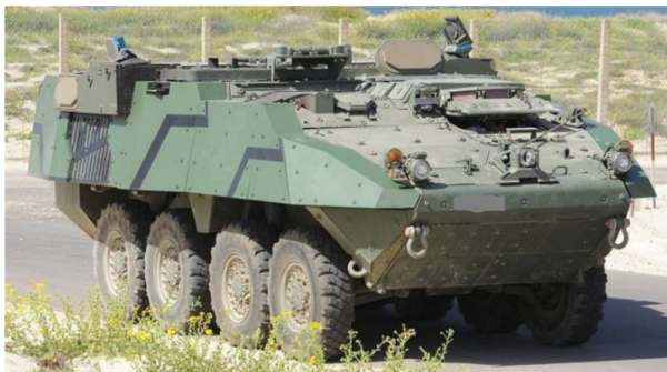
US Army Stryker equipped with Trophy, a real-world configuration that has undergone multiple tests (Rafael)
